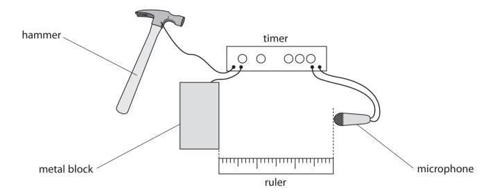
The student measures the distance between the front of the metal block and the microphone.
