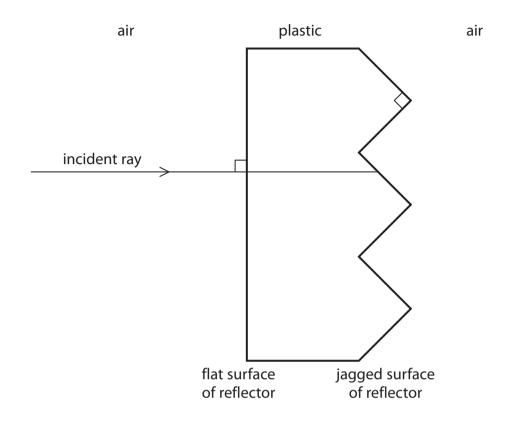
(i) The critical angle for the plastic of the reflector is less than 45°.
